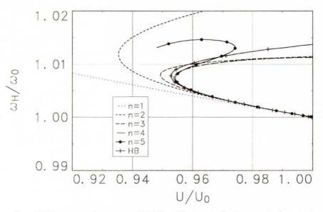
FIG. 10. Frequency of center-manifold Hopf limit cycle (antisymmetric flutter).
