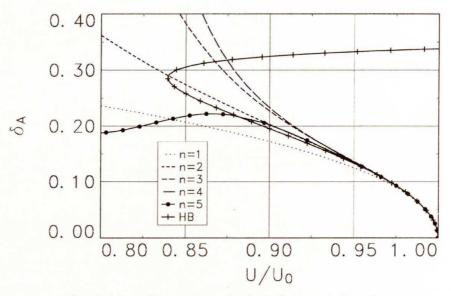
FIG. 8. Aileron limit cycle amplitude (antisymmetric flutter).
