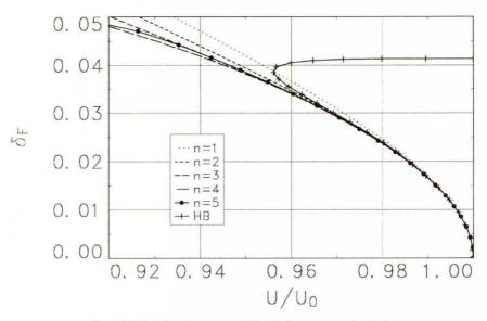
FIG. 3. Flap limit cycle amplitude (symmetric flutter).
