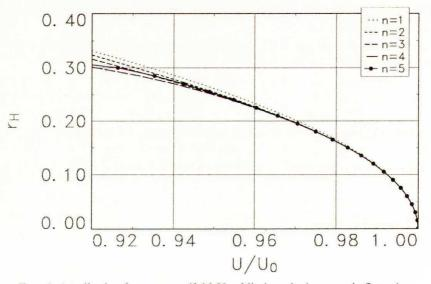
FIG. 1. Amplitude of center-manifold Hopf limit cycle (symmetric flutter).
