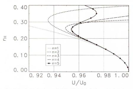
FIG. 9. Amplitude of center-manifold Hopf limit cycle (antisymmetric flutter).
