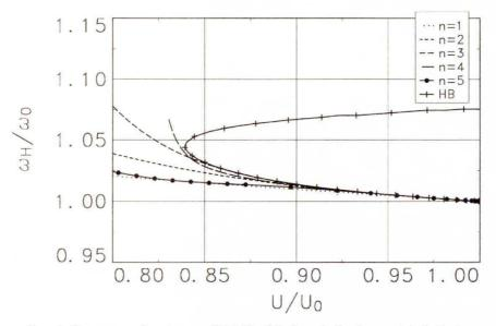
FIG. 6. Frequency of center-manifold Hopf limit cycle (antisymmetric flutter).
