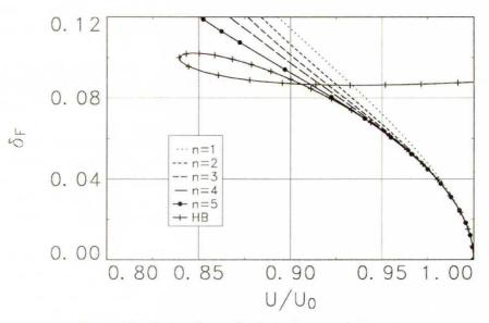
FIG. 7. Flap limit cycle amplitude (antisymmetric flutter).
