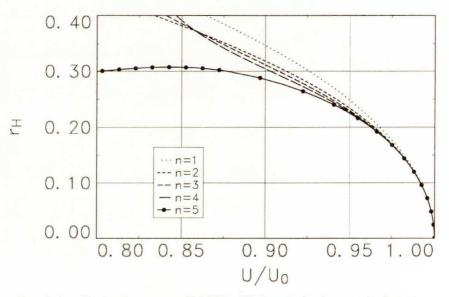
FIG. 5. Amplitude of center-manifold Hopf limit cycle (antisymmetric flutter).
