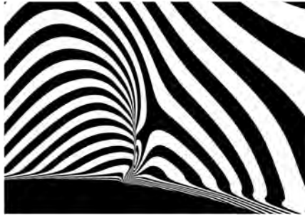
FIG. 6. Isolines of density 2D CFD, Ma = 1.26 , no control.
