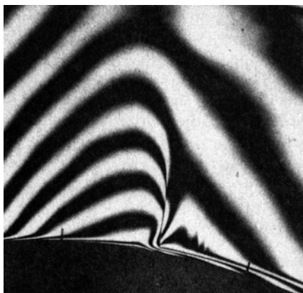
FIG. 3. Isolines of density Experiment, Ma = 1.26 , no control.
