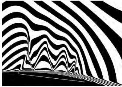
FIG. 7. Isolines of density 2D CFD, Ma = 1.26 , passive control.
