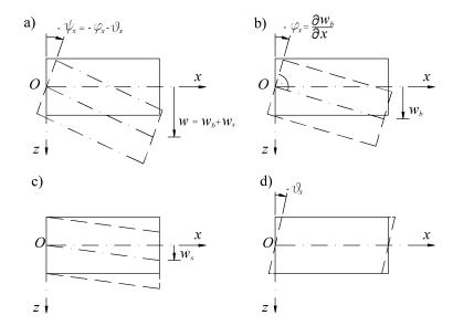
Fig. 2. Displacement components.
