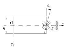
Fig. 3. Angular elastic support.
