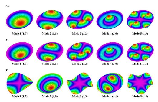
Fig. 4. The first five natural modes of simply supported (SS), clamped (C) and free (F) circular plate.
